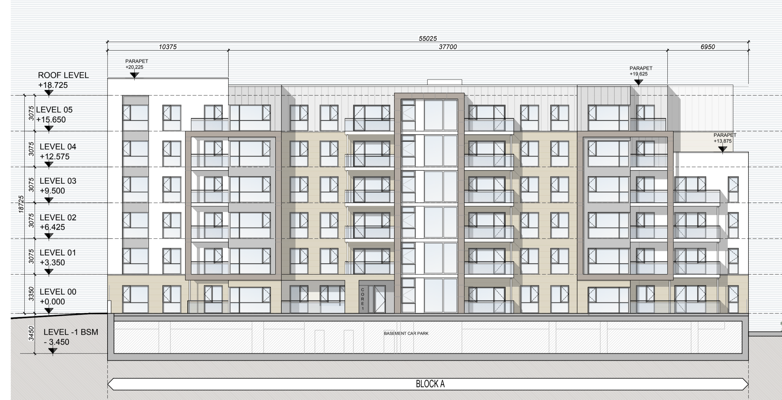
BLOCK A - EAST ELEVATION - 05
